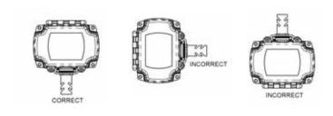
**FIGURE 2: OSA Mounting Orientation**
