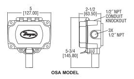
The Series WTP Wireless Temperature Sensors can be quickly installed on chilled water lines, air ducts or outside a building without having to run additional wiring. By sampling the temperature measurement every 10 seconds, the 3.6 V lithium battery is able to power the unit for up to 8 years.
