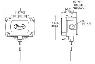
The Series WTP-R Wireless Remote Probe Temperature Sensors can be used to monitor surface temperature of water lines or in locations where space is limited. For greater flexibility, the enclosure for the electronics can be mounted up to 25′ from the temperature measurement point. By sampling the temperature measurement every 10 seconds, the 3.6V lithium battery is able to power the unit for up to 8 years.
