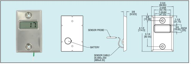
The Model WTI-100 Wall Plate Digital LCD Temperature Indicator is designed to display temperatures using an included remote thermistor. The easy to read LCD display is powered by a single CR2032 Lithium 3V battery. The wide operating range and SS wall plate allows the Model WTI-100 to monitor temperatures in walk-in freezers, indoor swimming pool areas, or general office environments.
