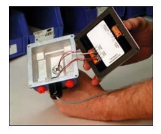
4. Add Electronics, Connect Wires
