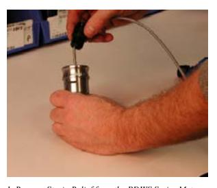
1. Remove Strain Relief from the PDWS Series Meter
