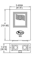
MODEL WA WATER LEAK DETECTOR offers affordable and dependable leak detection. This model is ideal for any application where a flood or water leak is likely to occur. It offers a loud audible alarm in the presence of water.
