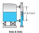
TYPICAL MEASUREMENTS C to C = L1 + 10.25" (260.35 mm) C to C = L1
