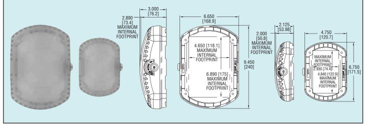
The Series TG Polycarbonate Thermostat Cover prevents physical damage and unauthorized adjustments of thermostats. Two sizes of covers are available to fit most common thermostats and transmitters. The low profile design with ventilation slits allows exceptional air flow in order to obtain accurate measurements. Each cover comes with two keys and mounting hardware for drywall and concrete walls. Model TG-1, Large Thermostat Cover Model TG-2, Small Thermostat Cover
