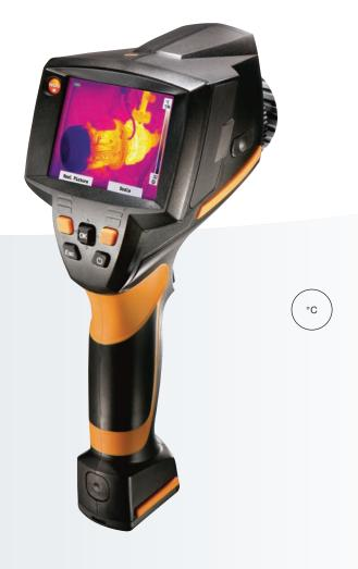
The thermal imager testo 875 quickly and reliably detects anomalies and weak spots in materials and components. Thanks to an imaging process, energy losses and cold bridges as well as damage or overheating in industrial systems are detected without contact. Whereas with other methods, cable or pipeline systems must be exposed over a large area, with the thermal imager testo 875, a single glance is enough.
