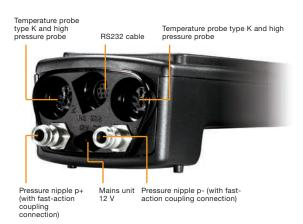
With the electronic differential pressure gauge testo 312-4, fine pressure measurements can be carried out quickly and reliably when checking the resting pressure and flow pressure of gas, and when setting the correct jet pressure on gas burners and boilers.
