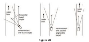
Small angles (less than 10°) have little effect on accuracy. As the angle increases, the displayed target velocity erroneously decreases, as Table 2 shows. At 90°, the target velocity is 0—grossly incorrect. Numbers such as these will be seen if the horizontal angle compensation option in the software menu is not set.
