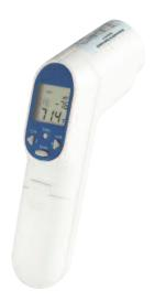
The Series IR3 Infrared Thermometer utilizes infrared technology for precise, non-contact temperature measurement. Models feature a 12:1 distance to target ratio and single point laser sighting for accurate temperature measurements. The IR3 offers an adjustable emissivity, backlit display, selectable temperature units, high/low alarms, minimum, maximum, differential and average functions.
