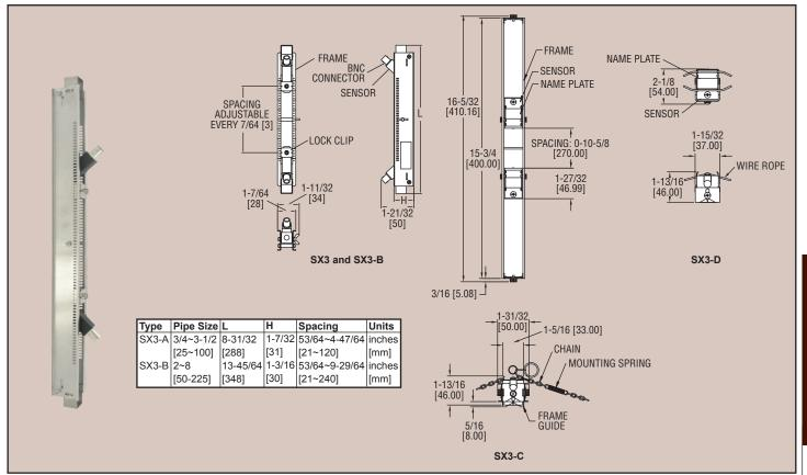
Series SX3 Ultrasonic Flowmeter Detectors are paired with Series UXF2 converters and employ a clamp-on type design for permanent use based on transit time measuring method. These detectors are ideal for clean liquids containing no air bubbles such as pure water. The easy-to-use compact and lightweight design is intended for integration into mechanical devices. It is applicable for small to medium size pipes of diameter range from 1 to 23 in (25 to 600 mm) and provides superior cost performance.
