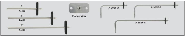
The Stainless Steel Static Pressure Tips are used to measure static pressures in ducts or rooms. They are to be connected to differential pressure switches and transmitters. Two static sensors are used in applications where differential pressure is required across a filter or coil. These sensors include a mounting flange with integral rubber gasket and two screws for simplifying mounting on a duct.
