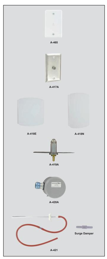
The A-465 Static Pressure Pick-Up provides a clean solution for sensing space pressure. The sensor can be mounted on sheetrock walls, single gang electrical boxes, or on ceiling tiles. Molded from ABS plastic, the A-465 provides an integral barb fitting and includes tubing, mounting screws and anchors.
