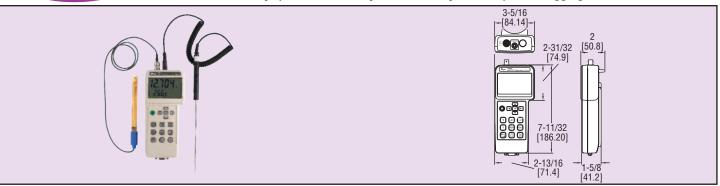
The microprocessor based pH/ORP/Temperature Meter offers quick response and high accuracy. Simultaneously measure and display pH from 0 to 14 pH (0 to 1999 mV) and temperatures up to 200°F (100°C). Model PHO-1 meter features manual or automatic temperature compensation, auto buffer recognition, and data logging capabilities, and the recording interval can be defined by the user. The Model PHO-1 accepts any pH electrode with a BNC connector.
