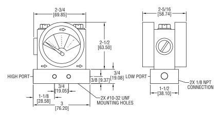
The Series PFG2 Process Filter Gage is designed for determining the state of an in-line filter. The differential pressure indicator determines the pressure drop on either side of a filter through its 1/8" female NPT pressure connections, and relates the value to one of three zones: clean (green), change (yellow), or dirty (red). The Series PFG2 is perfectly suited for filter applications, line loss, valve drop, and many other differential pressure applications where a simple indicator is needed.
