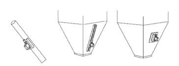
**Attention**: Vibration has to be fixed by a high tension bolt, washer, and spring washer. Connect with a security cable if the vibrator is installed onto a hopper.
