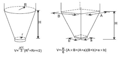
W: Material weight (KG) V: Chute volume (M<sup>3</sup>)
