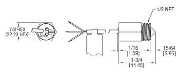
Compact and rugged this optical level switch provides rapid response while employing no moving parts for stable process control. The bright red and green LED's indicate the presence or absence of liquid for true, local indication. Three material options, 316SS, Polysulfone and PFA, provide application flexibility. Compact switch can be easily mounted horizontally or vertically.
