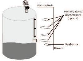
Figure 9: Scan Distance Process
