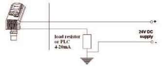
Figure 6: Non-Intrinsically Safe Negative Ground Connection
