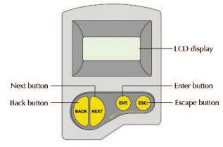
Figure 8: Display and Function Buttons
