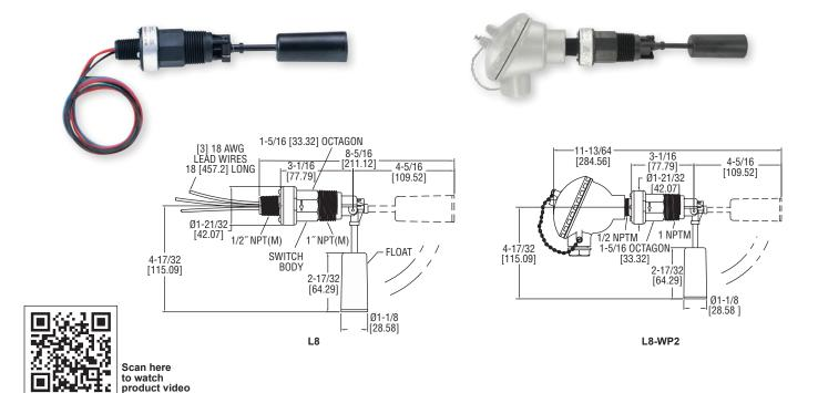
The **MODEL L8** Flotect<sup>®</sup> Liquid Level Float Switches is a float switch constructed of polyphenylene sulfide, Ceramic 8 and 316 SS. This liquid level switch provides accurate set point control of liquids with specific gravities as low as 0.6.
