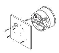
**B. SURFACE MOUNTING:** Drill (3) 3/16" dia. holes for mounting screws and (1) 7/8" dia. hole for wire assembly as shown in hole location drawing. Insert screws from rear of panel and thread into tapped holes on back of Photohelic® Switch/Gage case. If rear pressure connections are to be used, make 1/2" dia. holes located as shown in hole location drawing in left column.
