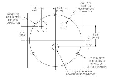
**4. MOUNTING:** The Photohelic® Switch/Gage may be either panel mounted or surface mounted.
