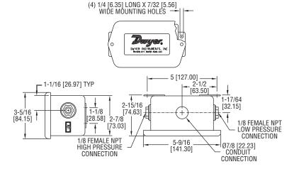
The Series 647 Wet/Wet Differential Pressure Transmitter is designed for use with compatible liquids or gases and can accurately measure differential pressure down to 1" H<sub>2</sub>O. The transmitter contains a fast response piezoresistive sensor and a unique isolation system ideal for HVAC systems, filter monitoring, variable speed drive control, air/liquid flow monitoring and process control.
