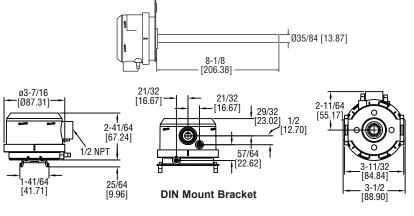
The Series MS Magnesense® Differential Pressure Transmitter is an extremely versatile transmitter for monitoring pressure and air velocity. This compact package is loaded with features such as: field selectable English or metric ranges, field upgradeable LCD display, adjustable dampening of output signal (with optional display) and the ability to select a square root output for use with pitot tubes and other similar flow sensors.
