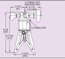
**Generate pressures** up to 10,000 psi (700 bar) with Model HHP-1 Hydraulic Hand Pump. Scissor action pump allows quick priming and pressure generation. Use in conjunction with an analog or digital pressure gage for a complete calibration system.
