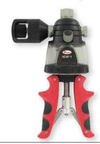
The **SERIES HCHP** Hydraulic Calibration Hand Pump utilizes a fully adjustable stroke control that allows for guick priming, easy pumping, and fast pressure generation up to 10.000 psi (700 bar). The ergonomically engineered handles provide extra comfort. while the triple filtration system ensures pump operation in spite of dirty conditions.
