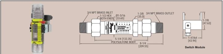
**Direct-Reading Series FS Flowmeters** offer visual flow rate indication in GPM or LPM units. Models include an adjustable, latching flow alarm to open or close AC electrical circuits, trigger warning lights, or activate other process control equipment. Spring-retained moveable piston design allows installation in any position.
