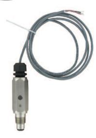
The Series TDFS is a thermal flow switch that indicates whether the flow rate is above or below a user set flow rate. The unit incorporates two LED status indicators providing visual switch indication. The set flow rate (setpoint) is field adjustable and the unit has both NO and NC NPN outputs. See Figure 1 for output and LED actions on change of flow.
