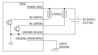
FIGURE 3: Wiring Diagram
