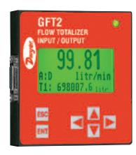
**The Series GFT2 Flow Totalizer** is a microcontroller driven device designed to linearize the flow meter and controller flow curve plus display the instantaneous flow rate, total, and accumulated total. The totalizer is intended to be used with analog flow meters and controllers with analog 0 to 5 VDC, 0 to 10 VDC, or 4 to 20 mA interface. RS-232 or RS-485 digital interface is available.
