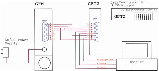
Figure 34: Connecting GFT2 to the GFM using 4-20mA output from DB9 connector.
