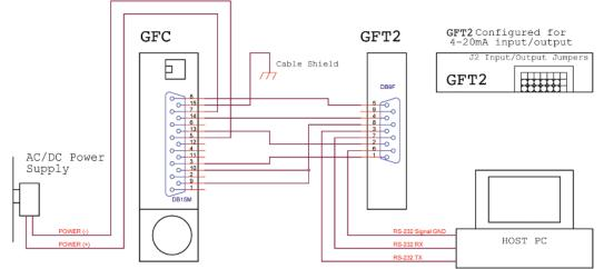
Figure 36: Connecting GFT2 to the GFC Using 4 to 20 mA Input/Output from DB15 Connector.
