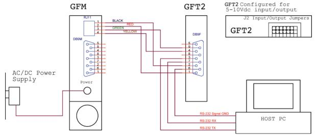
Figure 32: Connecting GFT2 to the GFM using 0-5 VDC output from DB9 connector
