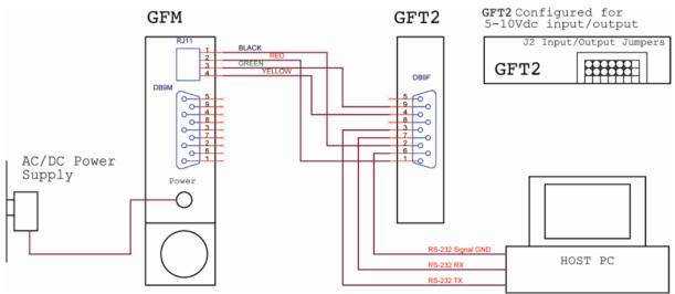
Figure 33: Connecting GFT2 to the GFM using 5-10 VDC output from RJ11 connector.
