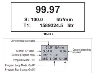
As shown in the above picture, the program run parameter can be toggled "On" and "Off" by pressing **RIGHT** and **LEFT** keypad buttons while PI screen 4 is active. If the Program Run status parameter set to "Off", the program execution will pause and current SP value will freeze until the Program Run status parameter is set to "On".
