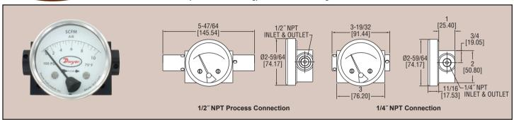
The Series DTFA Variable-Area Flowmeter for Gases measures gas flow rates with  $\pm 5\%$  of full-scale accuracy at an affordable price. Rugged aluminum construction ensures great compatibility and the strength to withstand system pressures of up to 3000 psig (200 bar). Available in either 1/4" or 1/2" NPT connections. Comes pre-calibrated for horizontal in-line mounting.
