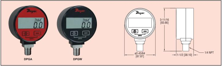
**The Series DPGA** is the only economic digital pressure gage with selectable engineering units on the market. With its 1% accuracy and digital push-button zero, the DPGA is the perfect choice for digitally monitoring the pressures of air and compatible gases.
