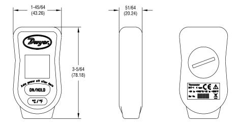
The Model DKT-1 Pocket-Size Thermocouple Thermometer accurately monitors temperatures in a variety of applications. The wide measurement range and selectable engineering units allow users to easily view readings in either °F or °C . The automatic power down feature conserves battery life. This compact thermometer accepts any K-type thermocouple sensors (sold separately) with
