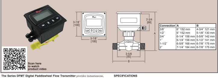
as well as totalizing flow monitoring, making it ideal for commercial and industrial systems. The large backlit LCD display makes navigating through the menu structure simple. The Series DFMT uses high accuracy paddlewheel technology, offers a user selectable 4 to 20 mA or pulse output, and has a corrosion resistant PVDF sensor giving it a long operation life. Users can reset the totalizer at any time and set a security password protecting the setting from unauthorized changes.
