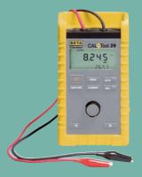
Consider the CALTool 20. With accuracy of  $\pm 0.015\%$ of reading and 0.001 mA resolution, the BETA CALTool 20 furnishes significantly extended performance over any competitive calibrator. A % Error function elimnates manual error calculations. The CALTool 20 simulates, powers and measures two-wire transmitters, and can remotely calibrate 4-20 mA devices.
