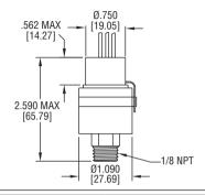
Miniature SERIES APS/AVS Adjustable Switches offer reliable switching for pressure/ vacuum alarm, shutdown or control. The units are readily adjustable throughout their range using the locking adjusting ring and indicating pointer. The body is constructed of stainless steel for durability in harsh environments. Switches include 12" (30 cm) wire leads sealed with epoxy for additional protection.
