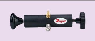
**Serves as pressure source** to calibrate gages and transmitters or to set pressure switches. Use with manometer or other pressure standard. Includes volume adjuster enabling fine pressure control and bleed valve. Generates pressures from a fraction of an in w.c. to 72 psig (5 bar). Includes barbed fitting, tee connector and three 36″ lengths of vinyl tubing.
