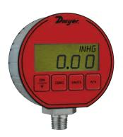
**The Series DPG-000 Digital Pressure Gage** has a precise +/-0.50% full scale accuracy. The 4 digit digital display will reduce the potential for errors in readings by eliminating parallax error commonly produced with analog gages.
