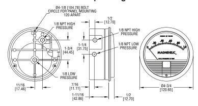
The Magnehelic<sup>®</sup> gage consists of two pressure-tight compartments separated by a molded flexible diaphragm.
