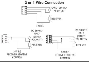
**CAUTION:** Do not exceed the specified supply voltage rating. Permanent damage not covered by the warranty may result. Do not use an external power source on the current loop connection.
