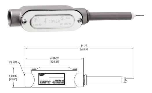
**The Series 641B Air Velocity Transmitter** uses a heated mass flow sensor technology. It has 4 user selectable ranges from 250 FPM to 2000 FPM with corresponding metric ranges of 1.25 MPS to 10 MPS. The 641B provides an isolated 4-20 mA output proportional to the velocity.
