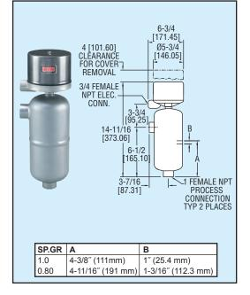
**Heavy duty and low cost** is the perfect description for the 391 Series level control. SS switching mechanism uses gravity return action instead of springs for long life. Weatherproof enclosure is standard. Welded steel chamber is good for 650 psig (45 bar) at 600°F (315°C).
