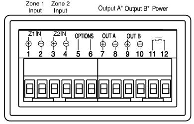
\* Output A is assigned to Zone 1 Input and Output B is assigned to Zone 2 Input. If necessary, the input/output relationships may be reversed. See 59 to in Secure Menu.
