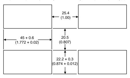
From the front of the panel, slide the housing through the cutout. The housing gasket should be flat against the housing flange before installing.
