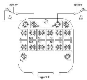
CAUTION: Do not apply electrical current to terminals in Sections B and C. Manual Reset with Circuit HH
