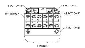
CAUTION: Do not apply electrical current to terminals in Sections B and C.
