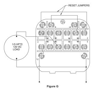
\*Note: For larger motors, use the Photohelic<sup>®</sup> in a maintained contact, 120 Volt Control or Push Button Circuit of the motor starter.
