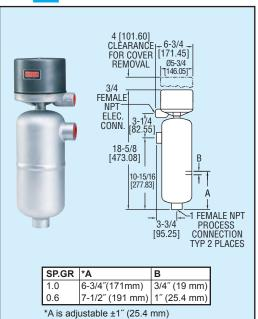
**Model 201 liquid level control** is designed for long life and reliable operation in chemical plants, refineries and industrial facilities. SS switching mechanism uses gravity return action instead of springs to prolong life. Weatherproof enclosure is standard. Heavy duty, welded steel float chamber is suitable for 500 psi at 750°F.
