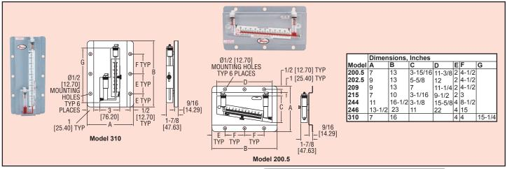
Dwyer® solid plastic stationary gages - or draft gages - are offered in inclined and vertical (well-type) styles for highly accurate laboratory or general industrial service, for measurement of low range gas and air pressures, positive, negative or differential. To assure the accuracy required in instruments of this type, all machining of bores and wells is to the highest standards of precision backed by Dwyer's years of experience in the fabrication of acrylic instruments.
