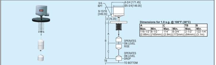
One of our most versatile level controls, the model B-190 can be used on all types of tank or sump level control applications. Three porcelain displacers provide deadband adjustment. Unit can start a sump pump (for example) when liquid reaches the high set point and turn the pump off when the level drops to the low set point. Unit works equally well in pressurized tanks. Two stage units also available.
