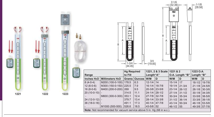
The SERIES 1221/1222/1223 Flex-Tube® U-Tube Manometer combines the inherent accuracy of the "U" Tube with the durability of tough, long-lasting plastic construction. The columns are made of 0.375" O.D. flexible and shatterproof clear butyrate tubing and are backed by a white scale channel to provide maximum color contrast. These manometers are ideal wherever a portable, direct reading manometer is needed.
