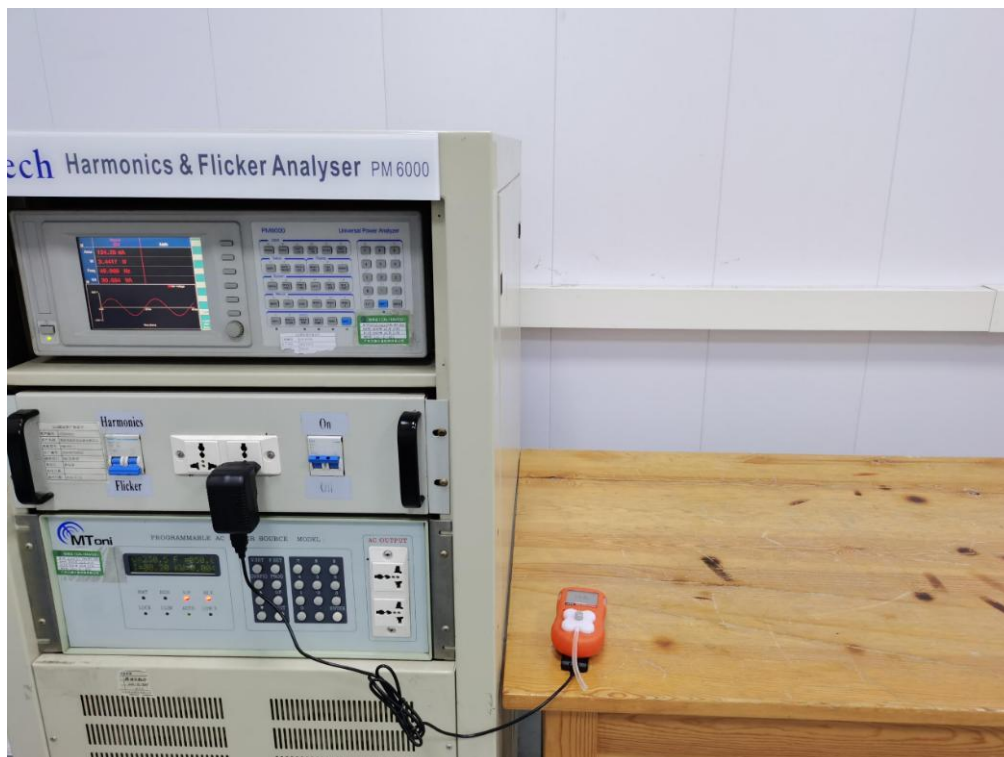
Test Setup Photo of Harmonic & Flicker Measurement
