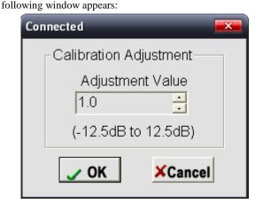
"Adjustment Value" is a Single calibration value, range: "-12.5" to "12.5", value "1.0" means "1dB".
