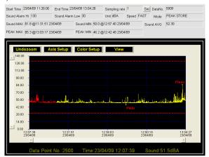
NORM MODE: Sound MAX/Sound MIN means the MAX degree or MIN degree of the sampling data. It is the average value of the 20 sampling data. PEAK MAX/PEAK MIN means the MAX or MIN degree of all the measuring values.(not the average value)
