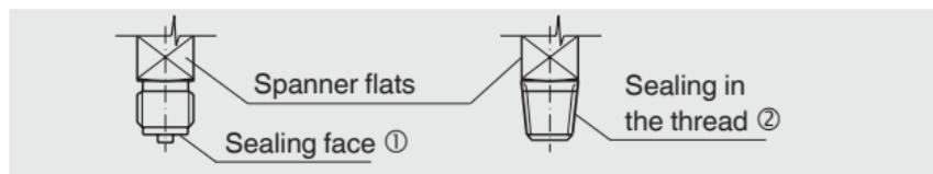
The torque depends on the seal used. Connecting the gauge using a clamp socket or a union nut is recommended, so that it is easier to orientate the gauge correctly. When a blow-out device is fitted to a
