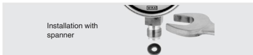
Correct sealing of pressure gauge connections with parallel threads ① must be made using suitable sealing rings, sealing washers or WIKA profile seals. The sealing of tapered threads (e.g. NPT threads) is made by providing the thread ② with additional sealing material such as, for example, PTFE tape (EN 837-2).
