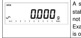
A stable sign ∼ is shown when the PMB is in stable condition. It will turn off if the reading is not stable. Exact zero is shown when the "→0← " symbol is on to the left of the display area.
