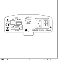
Attach the power supply cable to the connector on the rear of the analyzer. The master power switch is on the rear panel, next to the mains cable. Turn the power on.
