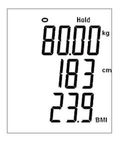
The results will remain on the display until the **[Clear]** key is pressed.
